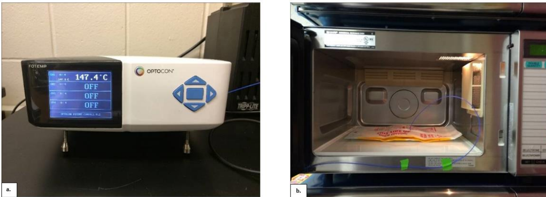
Figure 2.3. a.) Temperature probe reader used for temperature profiling; b.) Location of temperature probe in popcorn bag during cooking
